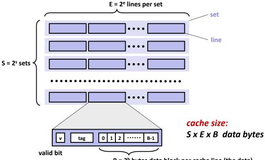
B = 2<sup>b</sup> bytes data block per cache line (the data)
