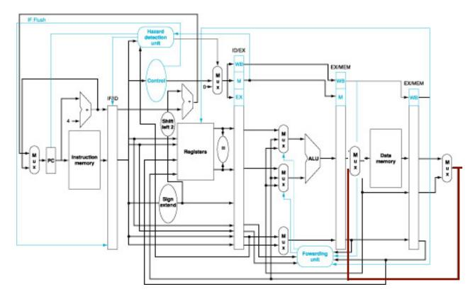
Note: alternatively you can assume no bypass, and instead insert stalls in the pipeline.
