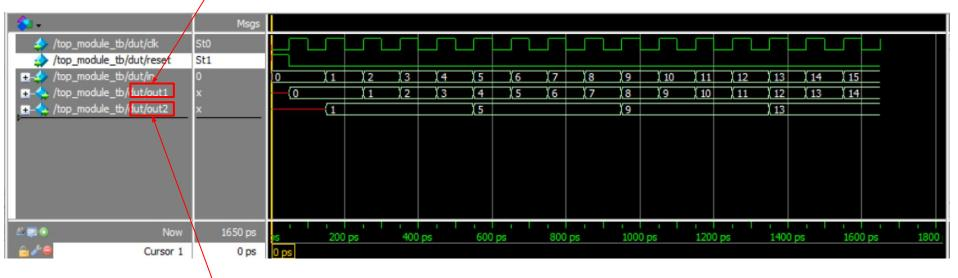
Output of the module A that does use divided clock (12.5 MHz clock)
