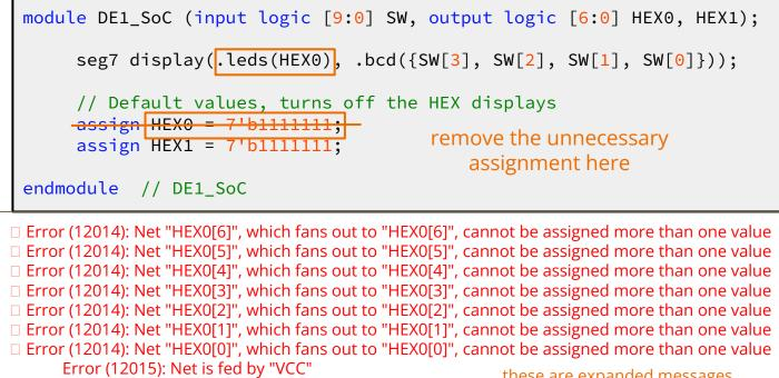
Error (12015): Net is fed by "seg7:display|leds[0]"
