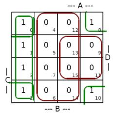
SoP:  $X = \overline{A} \overline{B} + \overline{B} \overline{D}$ PoS:  $X = (\overline{B})(\overline{A} + \overline{D})$
