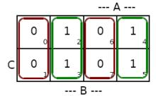
SoP:  $W = \overline{A}B + A\overline{B}$ PoS:  $W = (A + B)(\overline{A} + \overline{B})$
