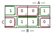
SoP:  $X = \overline{B}\overline{C} + BC$
