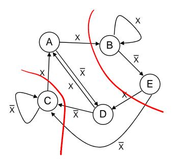
(b) Partition the FSM into *three* FSMs, one covering states A and D, another covering B and E, and the third covering C.
