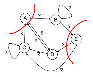
(a) Partition the FSM into two FSMs, one covering states A and E, and the other covering the remaining states.
