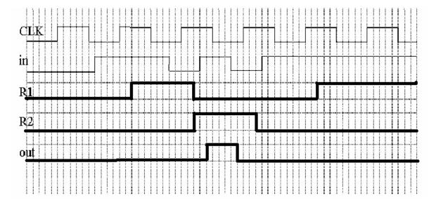
The original question had no set-up time listed which I corrected in class to 1 ns set-up time. Unfortunately, the signal into the second flip-flop did not respect this set-up time and transitions to high exactly on the 3<sup>rd</sup> positive clock edge. This means that it was also correct to have this signal ignored by the second flip-flop which would leave both R2 and out low throughout the time period. Such solutions also received full points.
