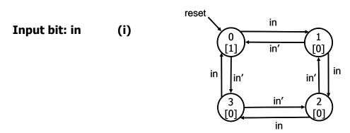
(ii) Encoding: State 0 = 00, State 1 = 01, State 2 = 11, State 3 = 10
