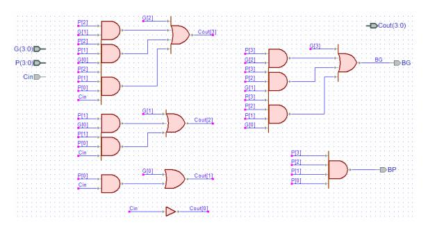
Note: BG is block generate, BP is block propagate.
