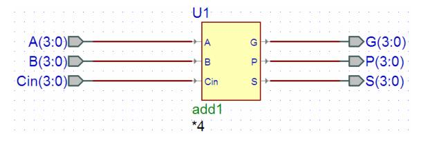
Note: This shows an implementation using vector notation. This could also be done without the vectoring, but the 4 1-bit adders must be independent of each other.
