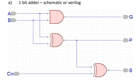
Note: Notice that propagate and generate signals are computed after 1 gate delay, and sum is computed 1 gate delay after the carry in is known.
