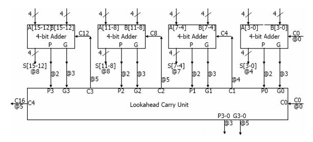
delay = (pi,gi calculation) + (P,G calculation) + (Block carry generation) +
