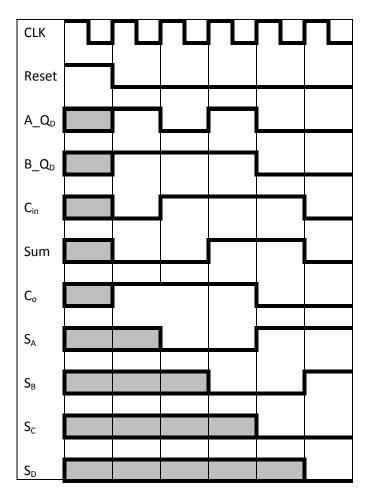
Notice that the sum is correctly calculated as 1100 (S<sub>A</sub>-S<sub>D</sub>) after four clock cycles (after reset).
