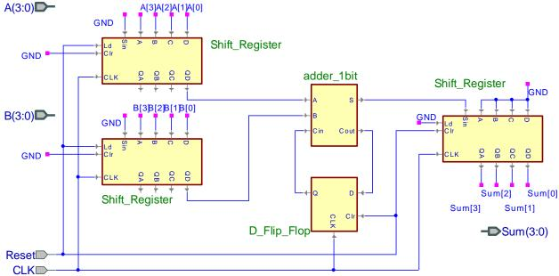
To handle the reset of the machine there are two things we need to do. First, we need to reset the carry flip-flop so that we start with no carry. Also, on reset we should do a "parallel load" of the A and B operand shift registers to load the initial values that we are adding. Some people had a separate load signal, this is okay.
