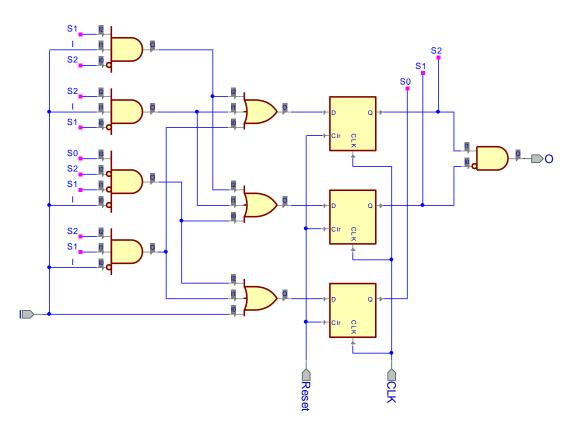
I have chosen to handle the reset signal by using flip-flops with a reset input. If our flip-flops do not have a reset input, then we can add an AND-gate to the input of each flip-flop such that the new value becomes:
