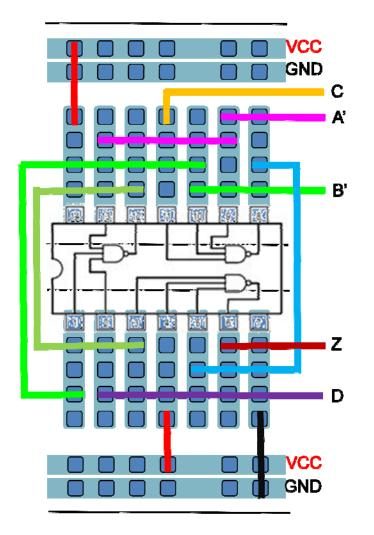
(c - 5pts) Assuming that '02 2-input NOR gates have a delay of 7ns and '10 3-input NAND gates have a delay of 9ns, what is the delay to Z of a change in an input (or its complement) for the circuit in part (a) and the circuit you wired up in part (b).
