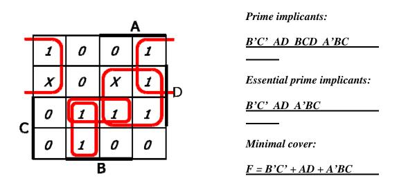
(b - 10 pts) Minimize the function  $G = \Pi M(1, 2, 5, 6, 12, 14) + D(0, 15)$  using the K-map below. List all prime implicants, essential prime implicants, and the minimal solution in SOP form in the spaces provided.
