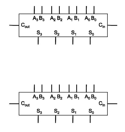
(c - 10 pts) If the delay of 4-bit adder of part (b) is 4 time units for the S bits and 3 time units for  $C_{out}$ , what is the delay of your implementation of the BCP adder (assume that all gates have a delay of 1). Make sure to explain how you derived your final delay for both  $C_{out}$  and the S outputs. Please highlight your result.
