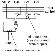
open-collèctor connection (zero whenever one connection is zero, one otherwise – wired AND)
