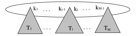
Children of each internal node are "between" the keys in that node. Suppose subtree  $T_i$  is the *i*th child of the node:
