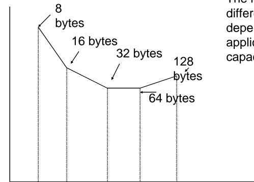
Typical form of the curve. The knee might appear for different block sizes depending on the application and the cache capacity
