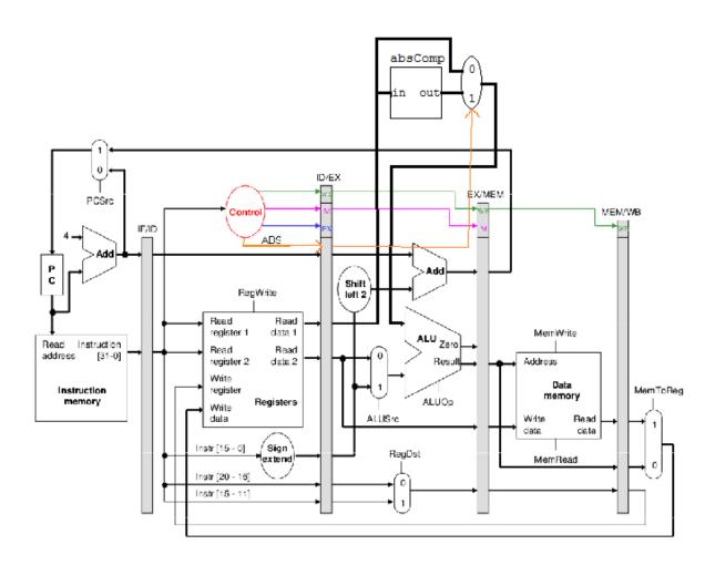
Note: This is only one of many possible solutions. All correct solutions involve adding the module, adding a multiplexer to choose between the module's output and the value of R[rs], and using a properly-forwarded ABS control line from the ID stage as the select for the added mux. It would also be ok to place the module between the ALU and the EX/MEM latch. In a real circuit, the best placement would need to take into account timing and delay issues, among other things.
