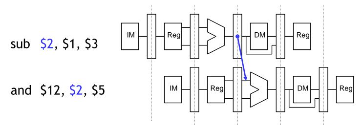
Data in a pipeline register can be referenced using a class-like syntax.
