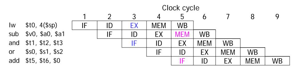
Thus, like the single-cycle datapath, a pipelined processor will need to duplicate hardware elements that are needed several times in the same clock cycle.
