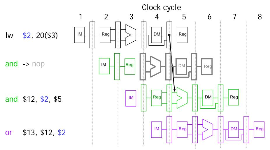
The effect of a load stall is to insert an empty or nop instruction into the pipeline
