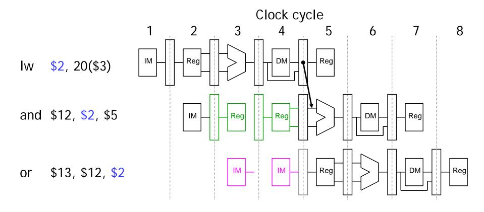
Those units aren't used in those cycles because of the stall, so we can set the EX, MEM and WB control signals to all 0s.
