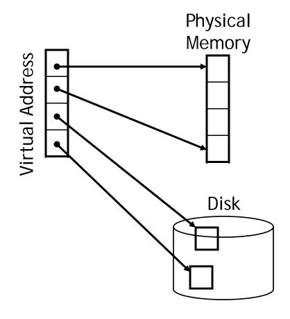
A virtual address can be mapped to either physical memory or disk.
