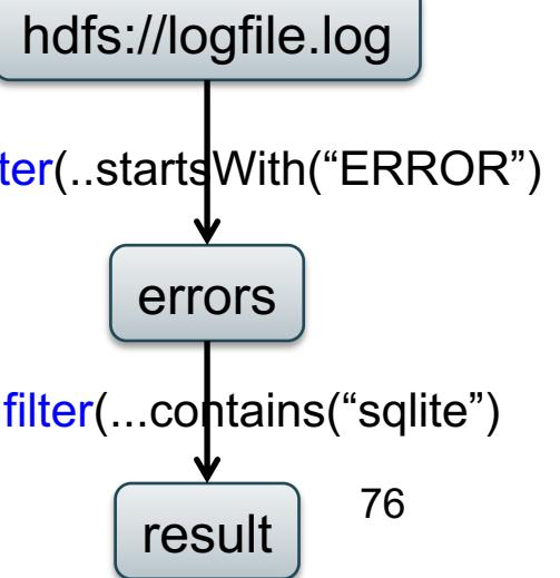
Spark can recompute the result from errors
