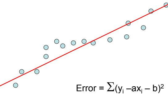
Determine set of K lines to minimize error
