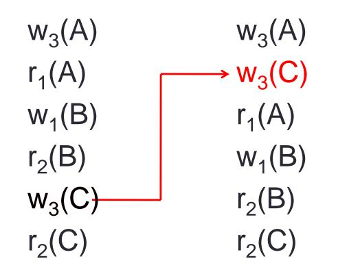
Only serial equivalent schedule: T<sub>3</sub>, T<sub>1</sub>, T<sub>2</sub>
