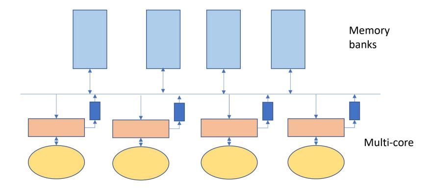
Suppose locations A and B start out with value 0. Core 0 writes 1 to A and then 1 to B, and no one else writes.
