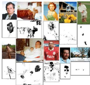
Figure 25.3. The figure shows a variety of images together with the output of the skin detector of Jones and Rehg applied to the image. Pixels marked black are skin pixels, and white are background. Notice that this process is relatively effective, and could certainly be used to focus attention on, say, faces and hands. Figure from "Statistical color models with application to skin detection," M.J. Jones and J. Rehg, Proc. Computer Vision and Pattern Recognition, 1999 © 1999, IEEE
