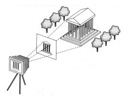
The image is rendered onto an **image plane** or **projection plane** (usually in front of the camera).
