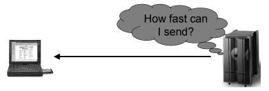
• Senders balance available and required bandwidths by probing network path and observing the response
