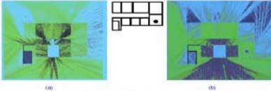
Fig. 4-1. Fluctuations of the electric field in the building that houses the faculty of Electrical Engineering. 2D FDTD code was used in these calculations which include the following: (a) all doors are open with no object present; (b) doors are closed with one object placed in one of the rooms. Green color denotes high electric field values, blue color represents low signal amplitudes.
