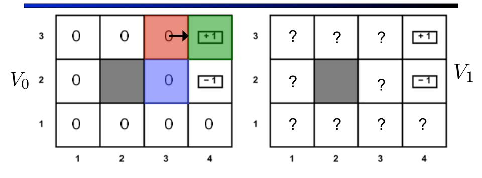
$V_{i+1}(s) = \max_{a} \sum_{s'} T(s, a, s') \left[ R(s, a, s') + \gamma V_i(s') \right] = \max_{a} Q_{i+1}(s, a)$  $Q_1(\langle 3, 3 \rangle, \text{right}) = \sum_{s'} T(\langle 3, 3 \rangle, \text{right}, s') \left[ R(\langle 3, 3 \rangle, \text{right}, s') + \gamma V_i(s') \right]$ = 0.8 \* [0.0 + 0.9 \* 1.0] + 0.1 \* [0.0 + 0.9 \* 0.0] + 0.1 \* [0.0 + 0.9 \* 0.0]
