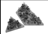
Fig. 1. Robots (programmable part) on an air table. Each edge of a part may attach to a square hole in another part. They attach by creating compression regions which disengage the table.
