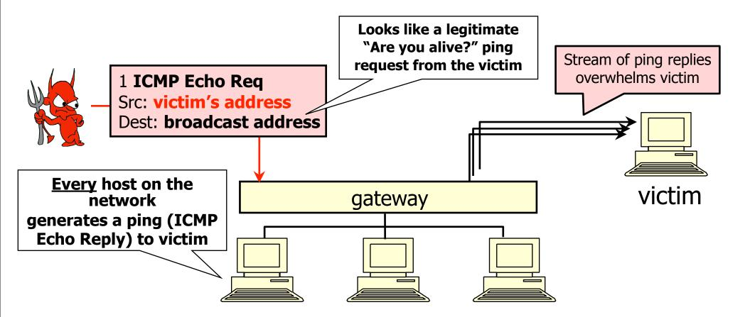
Solution: reject external packets to broadcast addresses
