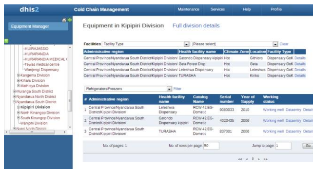
Figure 4 Screenshot of DHIS2 Cold Chain module showing a group of facilities and their associated refrigerators.
