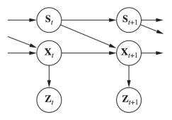
Figure 1: A Bayesian network representation of a switching Kalman filter. The switching variable  $S_t$  is a discrete state variable whose value determines the transition model of the continuous state variable  $X_t$ . For any discrete state *i*, the transition model  $P(X_{t+1}|X_t, S_t = i)$  is a linear Gaussian model, just as in a regular Kalman filter. The transition model for the discrete state  $P(S_{t+1}|S_t)$ , can be thought of as a matrix, as in a hidden Markov model.
