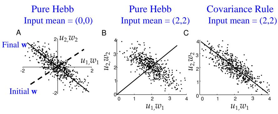
Hebb rule *rotates* weight vector to align with principal eigenvector of input correlation/covariance matrix (i.e. direction of maximum variance)
