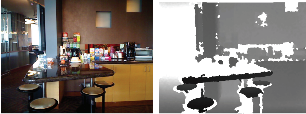
Fig. 1. (Left) RGB image and (right) depth information captured by an RGB-D camera. Recent systems can capture images at a resolution of up to 640 \times 480 pixels at 30 frames per second. White pixels in the right image have no depth value, mostly due to occlusion, distance, relative surface angle, or surface material.
