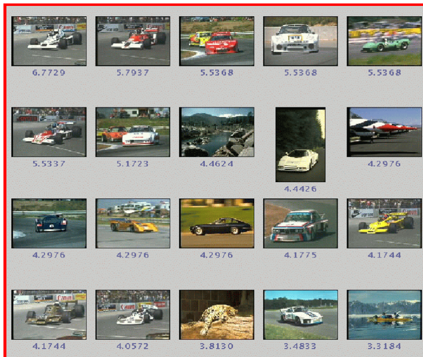
Figure 22.6. Querying using the “texture of textures” approach. The user has identified three pictures of cars as positive examples; these would respond strongly to large horizontal bar filters, among others. The system then chooses a collection of images at random (to represent irrelevant images); this data is then used to build a classifier to identify other images that are likely to be relevant. This query results in a number of returned images, containing several images of cars. Figure from “Boosting image retrieval” by K. Tieu and P. Viola, Proc. 2000 IEEE Computer Vision and Pattern Recognition © 2000, IEEE
