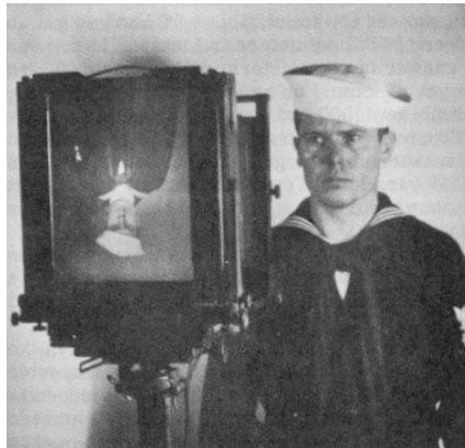
Figure 1.1. Image formation on the backplate of a photographic camera. Reprinted from [Navy, 1969], Figure 4-1.
