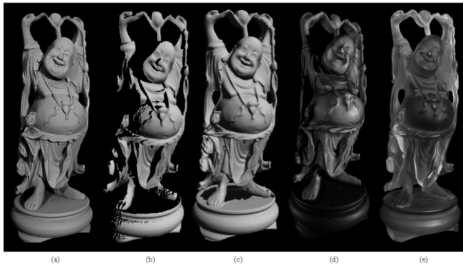
Figure 21.17. 3D Fax of a statuette of a Buddha. From left to right: photograph of the statuette; range image; integrated 3D model; model after hole filling; physical model obtained via stereolithography. Reprinted from [Curless and Levoy, 1996], Figure 10.
