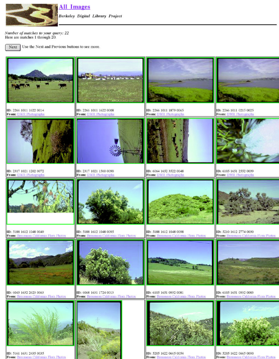
Figure 22.1. Results from a query to the Calphotos collection at U.C. Berkeley, that sought pastoral scenes. The query was composed by searching for images that contain many green and light blue pixels. As the results suggest, such colour histogram queries can be quite effective.
