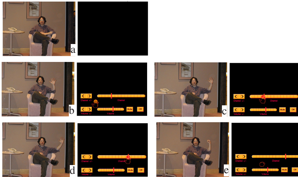
Figure 10.2. Examples of Freeman et al. 's system controlling a television set. Each state is illustrated with what the television sees on the left, and what the user sees on the right. In (a), the television is asleep, but a process is watching the user. An open hand causes the television to come on, and show its user interface panel (b). Focus on the panel tracks the movement of the user's open hand in (c), and the user can change channel by using this tracking to move an icon on the screen in (d). Finally, the user displays a closed hand in (e) to turn off the set.
