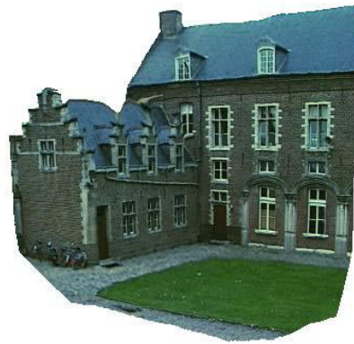
Figure 15.8. A synthetic texture-mapped image of a castle constructed via projective motion analysis followed by metric upgrade. The principal point is assumed to be known. Reprinted from [Pollefeys, 1999], Figure 6.13.
