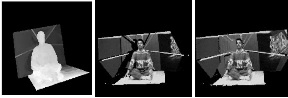
Figure 23.8. Multi-baseline stereo. From left to right: the range map associated with a cluster of cameras; a texture-mapped image of the corresponding mesh, observed from a different viewpoint; note the dark areas associated with depth discontinuities in the map; a texture-mapped image constructed from two adjacent camera clusters; note that the gaps have been filled. Reprinted from [Kanade and Narayanan, 1995], Figures 3 and 8.
