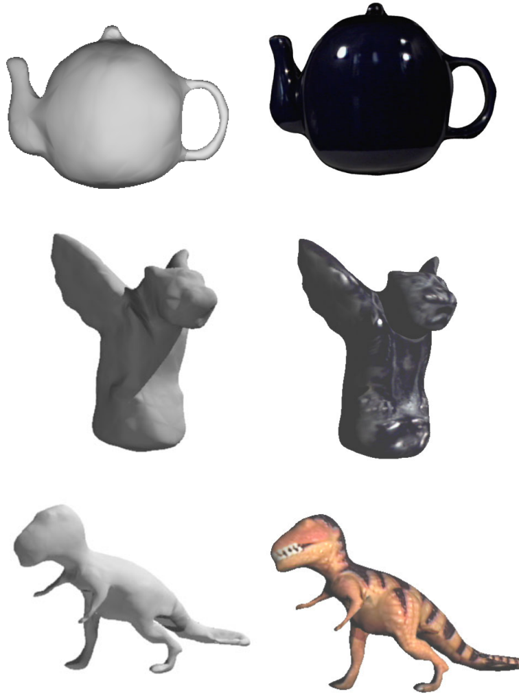
Figure 23.6. Shaded and texture-mapped models of a teapot, a gargoyle and a dinosaur. The teapot was constructed from six registered photographs; the gargoyle and the dinosaur models were each built from nine images. Reprinted from [Sullivan and Ponce, 1998b], Figures 4 and 5.
