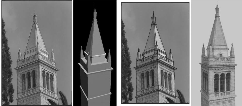
Figure 23.10. Façade model of the Berkeley Campanile. From left to right: a photograph of the Campanile, with selected edges overlaid; the 3D model recovered by photogrammetric modeling; reprojection of the models into the photograph; a texture-mapped view of the model. Reprinted from [Debevec et al. , 1996], Figure 2.
