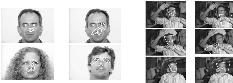
Figure 26.5. Perona et al. 's face detector looks for local patterns, which are classified on their appearance using filter responses. Appropriate arrangements of these patterns are faces. Relations between face points are represented by the inter-element distances, and the class-conditional density for these distances is gaussian. In turn, this means that, once some feature responses have been found, the position of others can be predicted. The figure on the left illustrates predictions for different feature points. The features are points around the eyes, nose and mouth, and the variation in inter-point distances comes from individual variations in facial structure. The figure on the right illustrates the behaviour of the overall face detector; the column on the left shows the best face in the image, and the column in the right shows the second best, which typically has a posterior value that is smaller by an order of magnitude. Figure from, "Finding faces in cluttered scenes using random labelled graph matching," by Leung, T. ;Burl, M and Perona, P., Proc. Int. Conf. on Computer Vision, 1995 © 1995, IEEE
