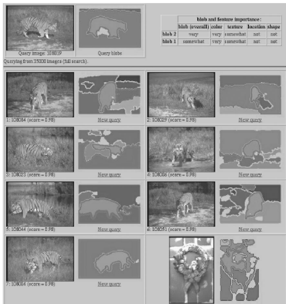
Fig. 7. Blobworld query for tiger images using two blobs. The overall weights are 1.0 for the tiger blob and 0.5 for the grass blob. For both blobs, the color weight is 1.0 and the texture weight is 0.5.
