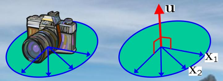
Up-vector perpendicular to plane of camera x vectors
