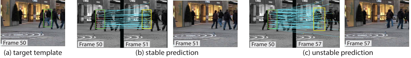
Figure 3. The appearance of the target is represented by a template in a video frame (a). We compute optical flow from densely sampled points inside the target template to a new frame. The quality of the flow is used as a cue to make the decision: (b) an example of stable prediction; (c) an example of unstable prediction due to partial occlusion, where we show both the cropped frames and the origin frames. The yellow box is the predicted location of the target.
