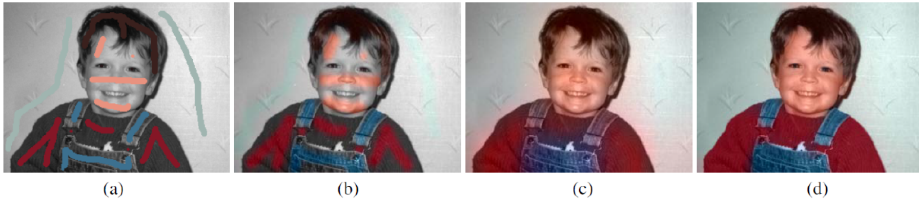
Figure 4.12 Speeding up the inhomogeneous least squares colorization solver using locally adapted hierarchical basis preconditioning (Szeliski 2006b) © 2006 ACM: (a) input gray image with color strokes overlaid; (b) solution after 20 iterations of conjugate gradient; (c) using 1 iteration of hierarchical basis function preconditioning; (d) using 1 iteration of locally adapted hierarchical basis functions.
