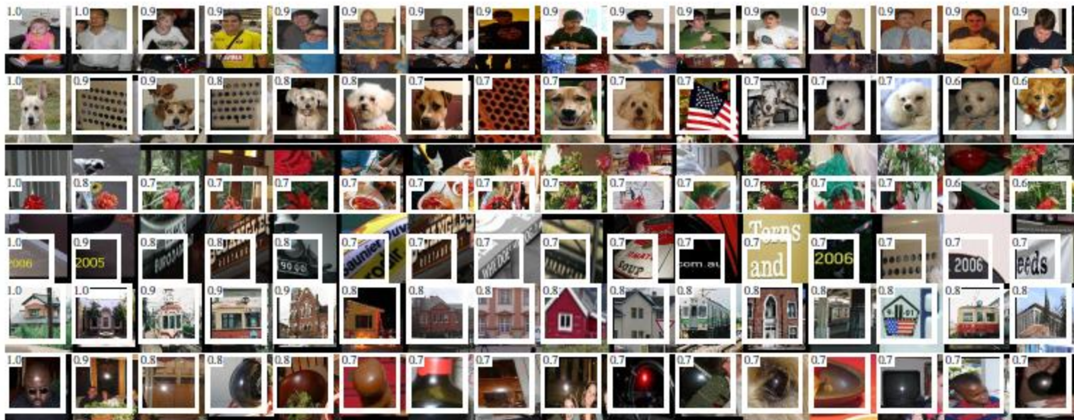
Figure 4: Top regions for six pool 5 units. Receptive fields and activation values are drawn in white. Some units are aligned to concepts, such as people (row 1) or text (4). Other units capture texture and material properties, such as dot arrays (2) and specular reflections (6).
