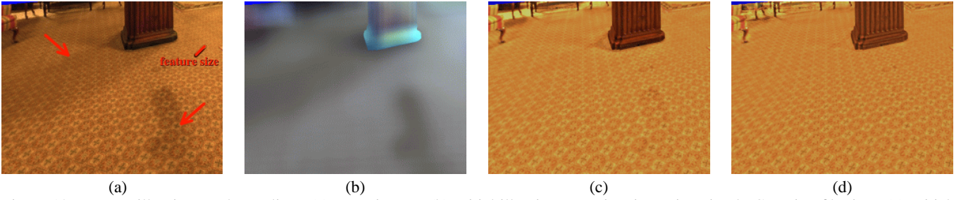
Figure 10: Texture-illumination decoupling. (a) Input image. (b) Initial illumination estimation using simple Gaussian filtering. (c) Initial texture estimation, note the artifacts corresponding to shadow boundaries. (d) Texture computed using bilateral filtering.
