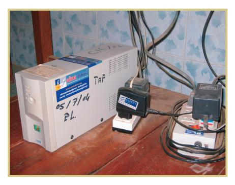
Heat is the next obvious problem. In developing regions, equipment must operate in a wide range of temperatures because of the lack of widespread climate control. Although cooling the rooms containing computers is sometimes possible, doing so is expensive and requires power, and cooling systems are unlikely to be handled by a UPS (uninterruptible power source).
