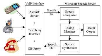
Fig. 3. Block diagram of HealthLine system components.
