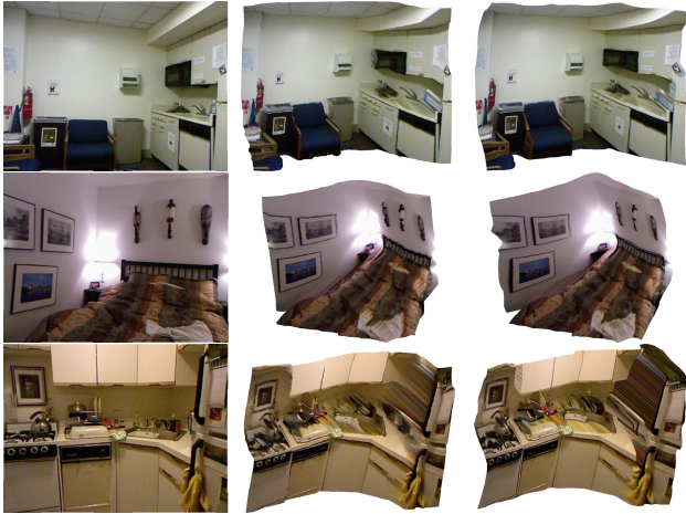
Figure 5. After a model is recovered, the camera can be moved and the input image (left) can be shown from a different viewpoint (right). Such a warping could be produced using just the smoothed Kinect depth maps provided in the NYU dataset (middle), but these images have jagged artifacts at surface and normal discontinuities. Both renderings, of course, contain artifacts in occluded regions.
