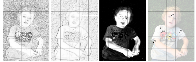
Figure 3. Our features. Far left: Each cell is HOG with local gradient contours. Left: Each cell is HOG with gPb. Right: We compute the average value of the skin classifier at each cell. Far right: Our context feature; at each cell we have a poselet activation feature vector. For each poselet type, we put the maximum of the scores of all poselet activations of that type whose center falls in the cell, or zero if no activations are present.
