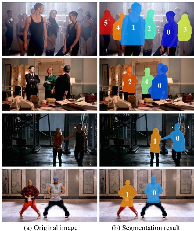
(a) Original image (b) Segmentation result Figure 5. Qualitative results on images from the movie “Street-Dance”. Each row shows the original image and the corresponding segmentation. Rows 1 and 2 demonstrate successful handling of occlusion between several people. The method can also handle non-trivial poses, as shown by Rows 3 and 4. The segmentation results are generally accurate, although some inaccuracies still remain on difficult examples. For instance, in Row 1, the segmentation is leaking into background for persons 3 and 5, due to the weak disparity cue for these people far away from the camera. The numbers denote the front (low values) to back (high values) ordering of people. (Best viewed in colour.)
