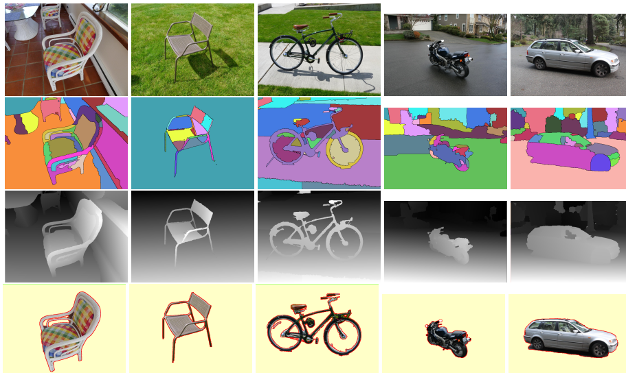
Fig. 5: [ COLUMNS 1 – 5] Results on CHAIR1, CHAIR2, BICYCLE, BIKE and CAR sequences respectively. [Row 1-3] A sample image from each dataset is shown along with its piecewise-planar surface labeling and the corresponding depth-map computed by our method. [Row 4] The final segmentations recovered by our method. Notice how thin structures and holes in objects with complex topologies are accurately segmented (see columns 1–3). Our method accurately deals with camouflage where the object and background colors are similar (see columns 4 and 5), and is also robust to the presence of strong specularities and reflections (see column 5).
