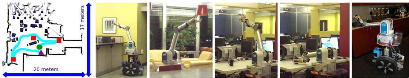
Fig. 14 (Color online) Map of the kitchen environment used for fetch tasks (left). Herb starts at the green circle and generates a path to look for a coffee mug at the locations marked by red squares . After finding
