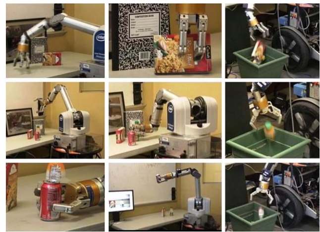
Fig. 13 Snapshots from three runs of the planner on the WAM arm. Top Row: Grasping and throwing away a box of rice. Middle Row: Grasping and throwing away a juice bottle. Bottom Row: Grasping and throwing away a soda can
