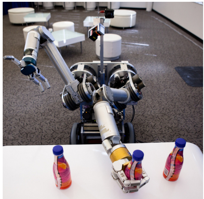
Fig. 1. HERB 2.0: A bimanual mobile manipulator developed at the Personal Robotics Lab at Carnegie Mellon University
