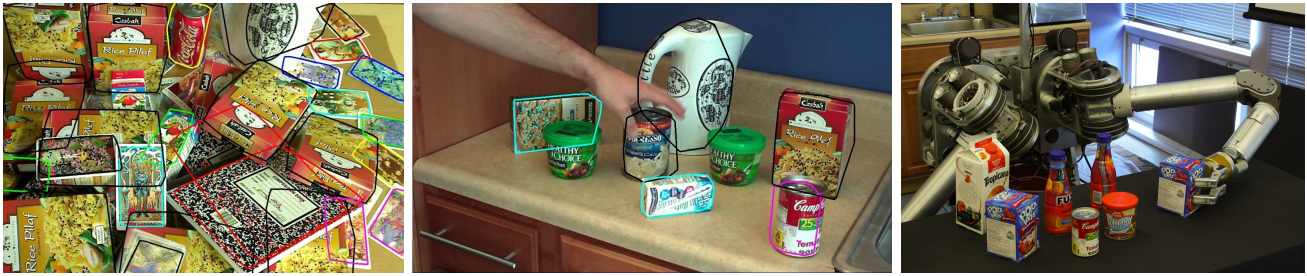
Fig. 9. Recognition of real-world scenes. (Left) High-complexity scene. MOPED finds 27 objects, including partially-occluded, repeated and non-planar objects. Using a database of 91 models and an image resolution of 1600 \times 1200 , MOPED processes this image in 2.1 seconds. (Middle) Medium complexity scene. MOPED processes this 640 \times 360 image in 87 ms and finds all known objects (The undetected green soup can is not in the database). (Right) HERB 2.0 grasping object recognized and registered by MOPED. Images taken from [68].
