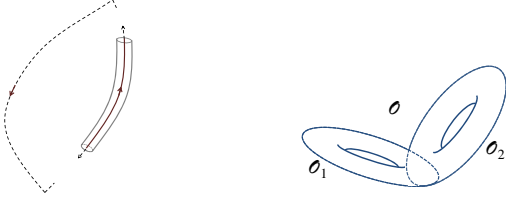
(a) An unbounded obstacle and its skeleton can be closed at a large distance to create a closed loop. (b) An obstacle with genus 2, \mathcal{O} , can be decomposed into 2 obstacles, each with genus one, \mathcal{O}_1 and \mathcal{O}_2 .
