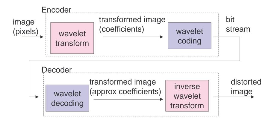
A wavelet transform decomposes the image into a low resolution version and details. The details are typically very small so they can be coded in very few bits.
